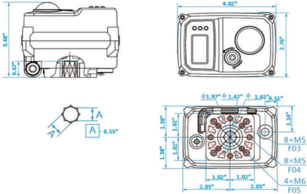
**PART NUMBERS S20.26 133in.lbs SMART FAILSAFE MODULATING ACTUATOR**
